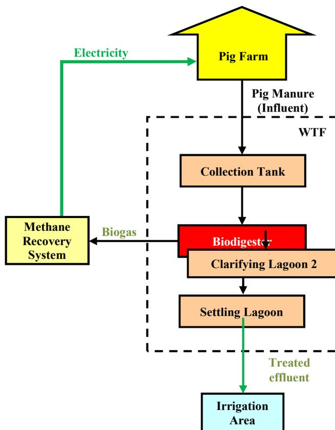
Figure 3. Wastewater treatment and power generation process of CPA 34
