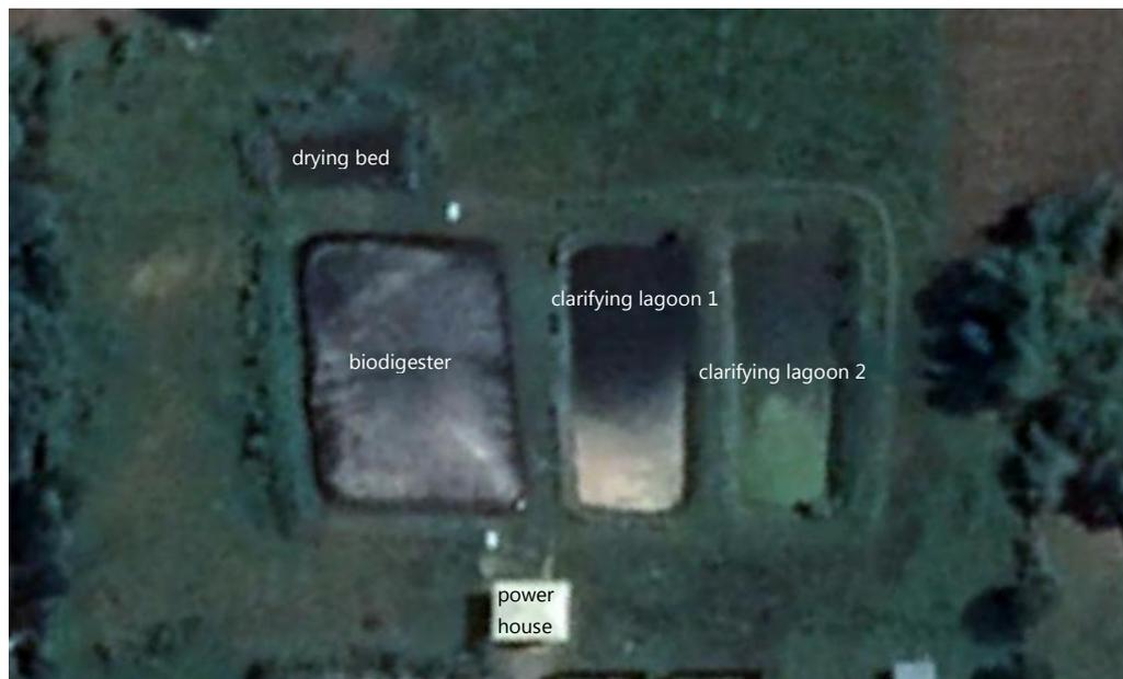
Figure 3. Satellite image of GREG III Farm's Wastewater Treatment Facility (Image generated using Google Earth<sup>®</sup>)
