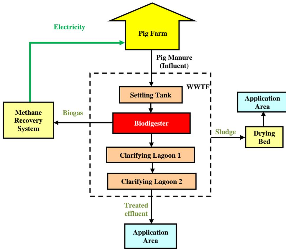
Figure 2. Wastewater treatment process of GREG III Farm
