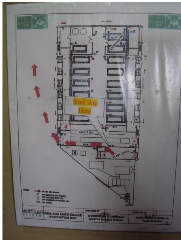
Figure 20. Evacuation map showing the exit routes and locations of fire extinguishers
